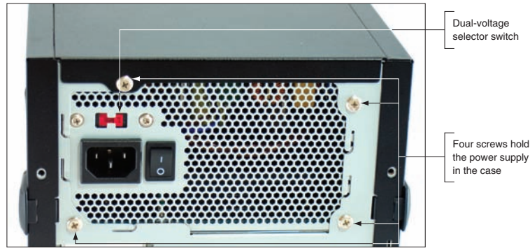
Figure 1-21 The dual-voltage selector switch sets the input voltage to the power supply
